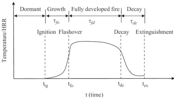
Fig. 2: The phases of enclosure fire development [3]
