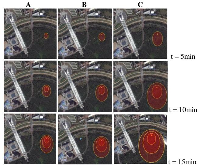
Fig. 7: Results of fire spread simulation. (A)  $V = 3$  m/s, (B)  $V = 12$  m/s, (C)  $V = 24$  m/s
